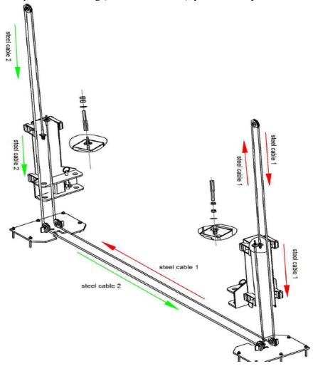
Step 7: Put the power unit on the post
